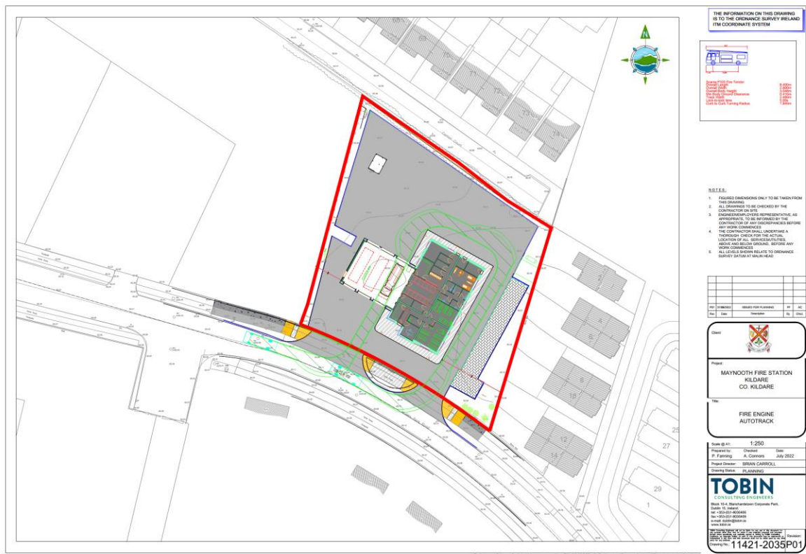
Figure 3-1: Fire Engine Swept Path Analysis, 11421-2035
